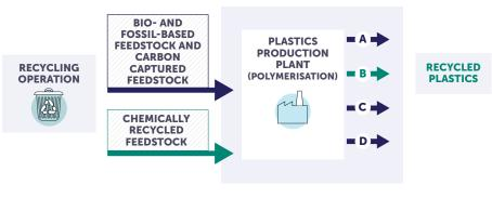
Mass balance allows the attribution of recycled characteristic, to one or several outputs products.
